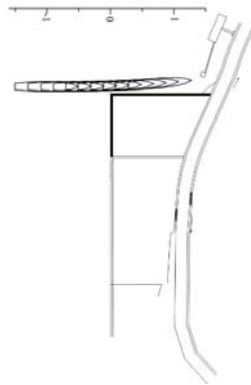
Fig. 6. Result of simulation under the influence of bank effect ( S_p = 0.1L , \delta = 0^\circ ).
